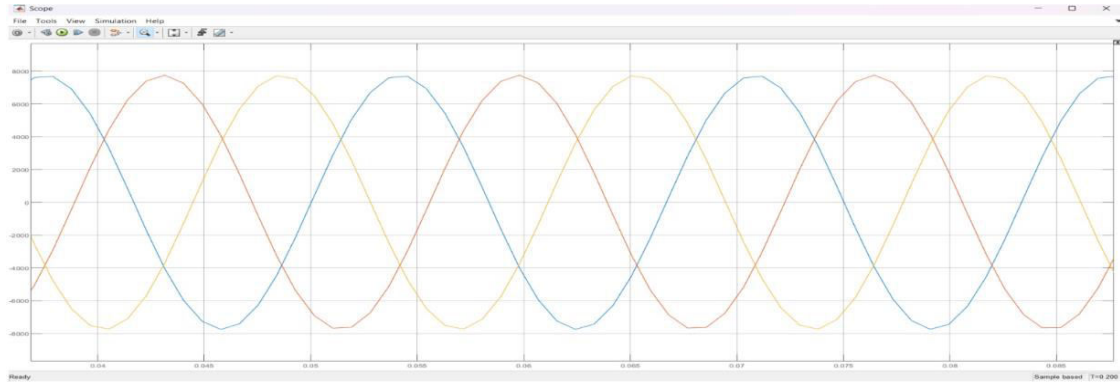
Fig.5. Three-Phase Voltage Waveforms from Simulink Scope
